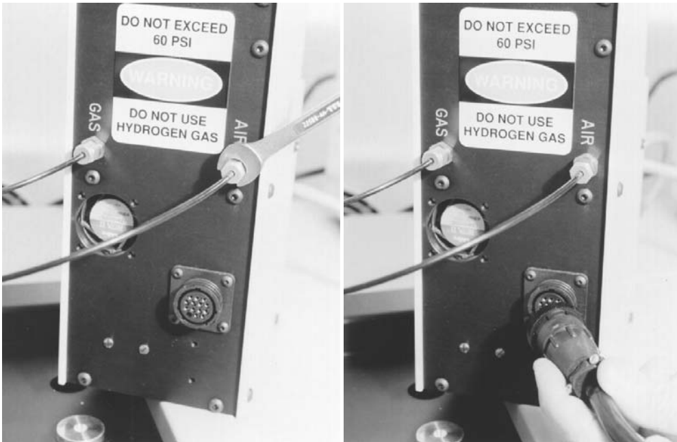
Figure 2-8 – (a) 1/8" Teflon™ tubing is used for the carrier gas line and the compressed air line on the Desorption Unit; (b) Installation for the interconnect cable (#782010).
