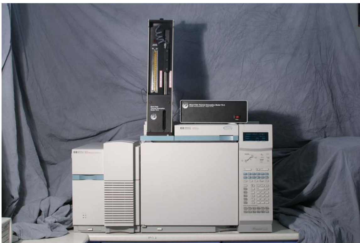
Figure 2-9 – TD-5 Desorption Unit installed on the Agilent 6890 injection port. Electronics Console is shown to its side (but may be placed elsewhere).
