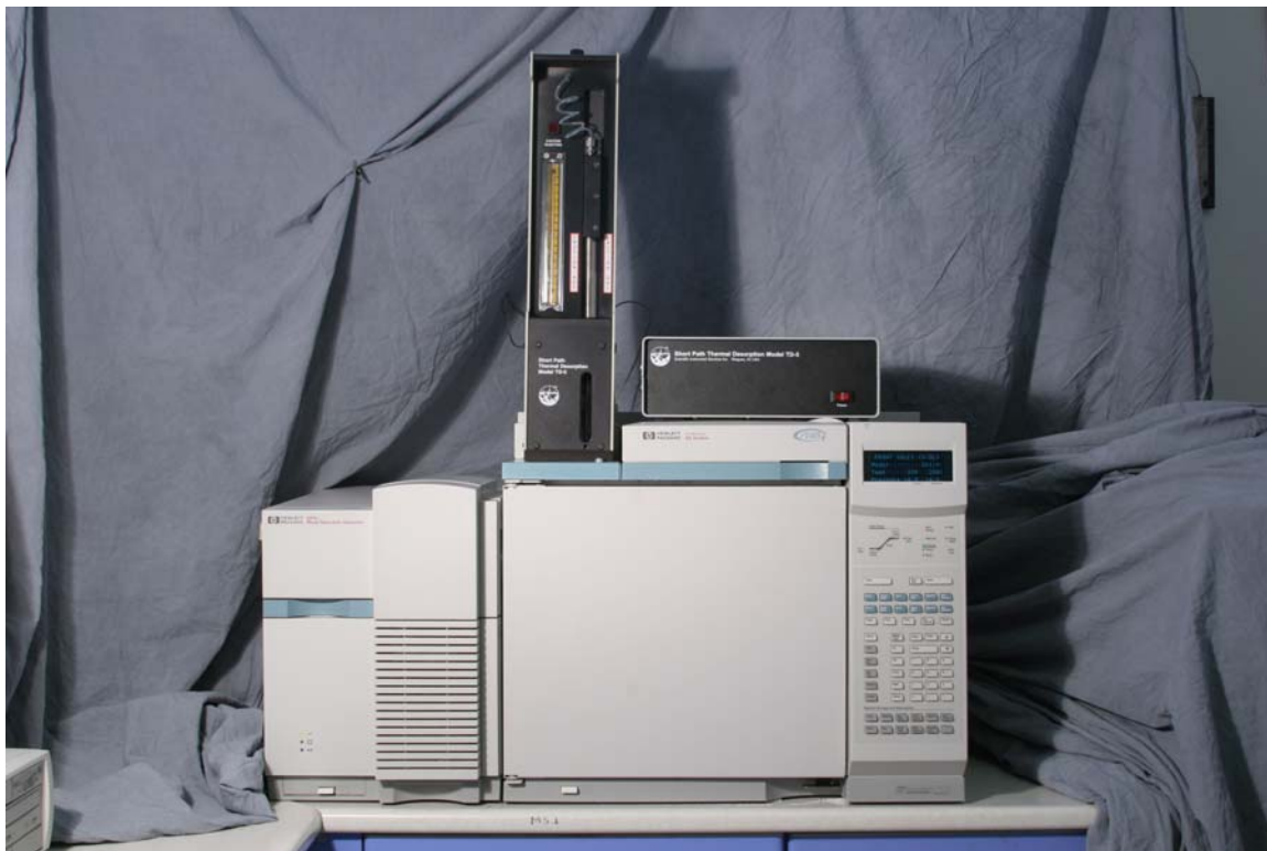
Figure 1-8 – SIS TD-5 system installed on a GC (Agilent 6890 GC shown here).
