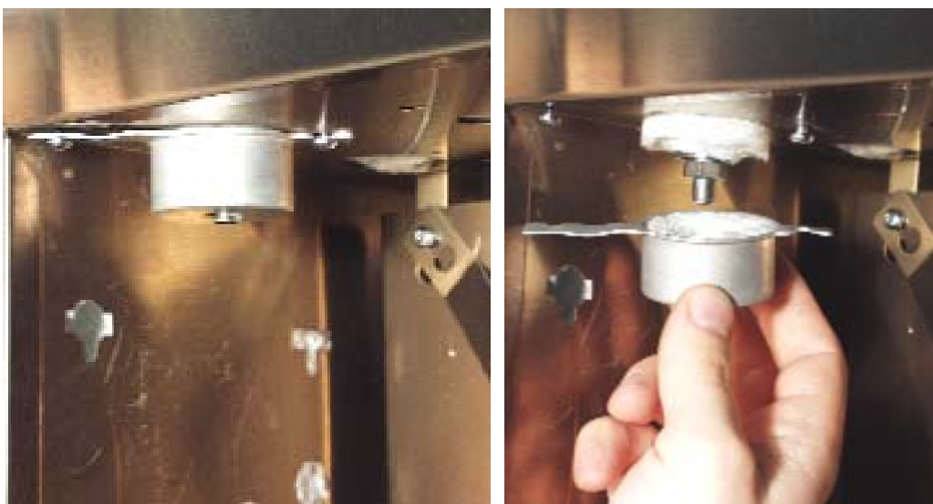
Figure 2-11 – Remove insulation cup from inlet
